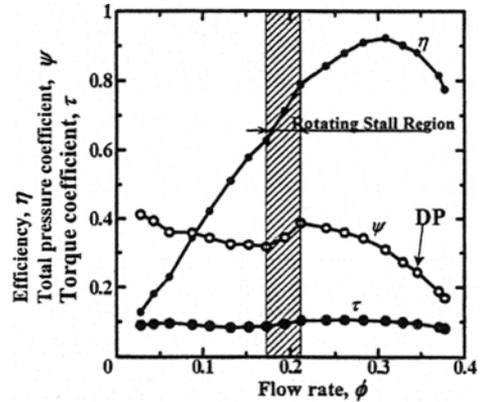
**Fig. 2** Characteristic curves of test fan
